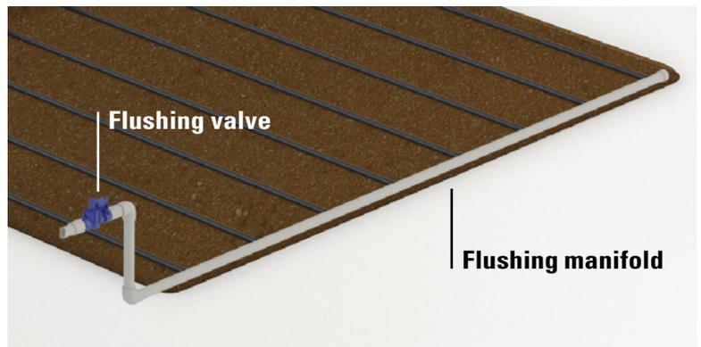
The flushing manifold is sized for a flow velocity of at least 0.5 m/sec (1.65 ft/sec) at the end of the dripperlines to ensure sediment removal.
