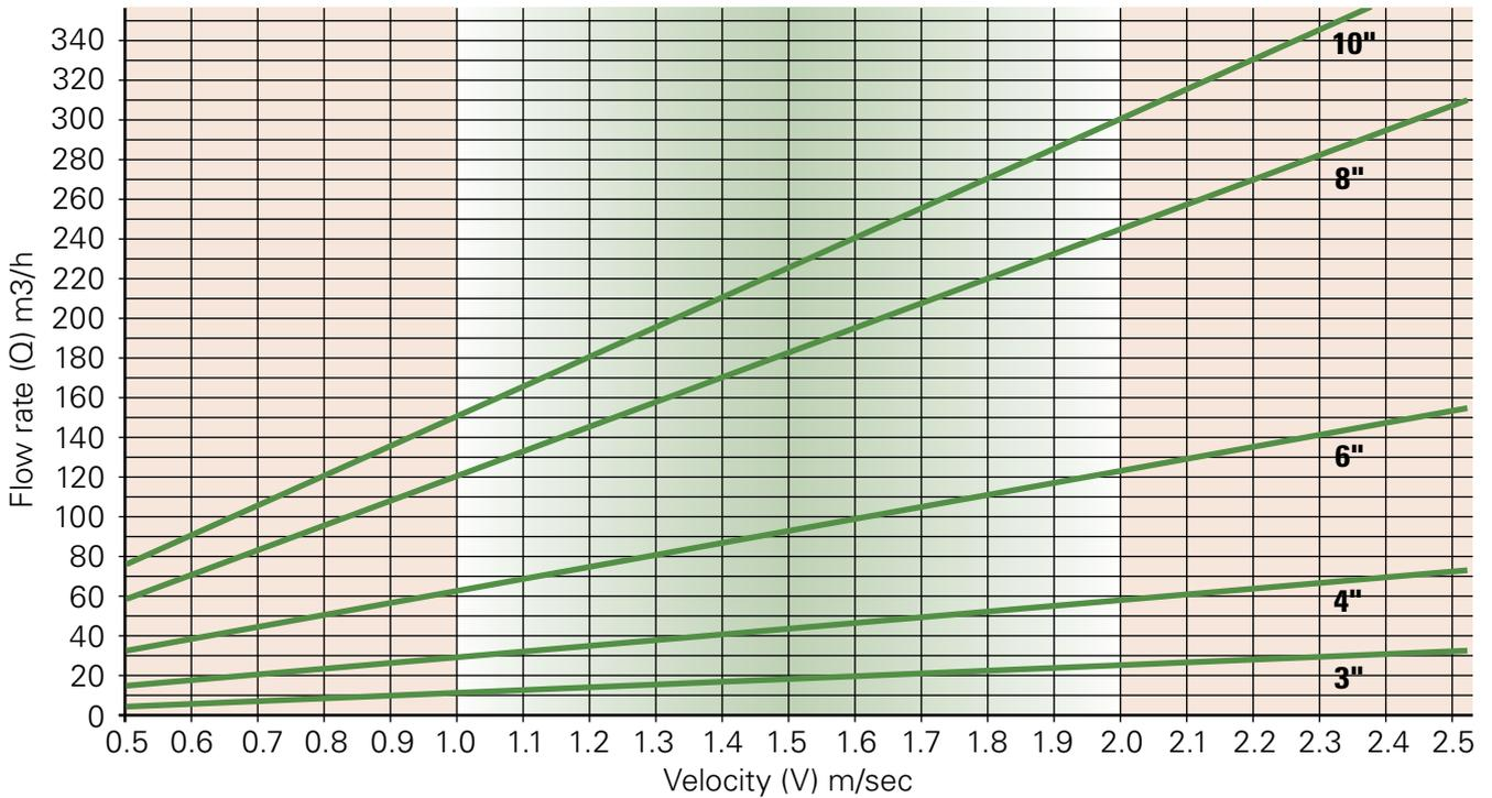
\* The graph represents the velocities in pipes of one specific standard among many. If the pipe used in the system's main, sub-main or distribution lines does not appear in the above table and graph, find the actual internal diameter of the pipe in the pipe documentation and calculate the velocity using the following formulas:
